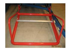
For loading of small bales a tube mounted on the loading grab makes it possible to lift small bales onto the bale wagon. The tube can be mounted in different positions on the loading grab.
